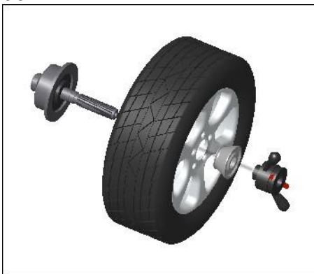
Main shaft--wheel (Installing face of rim forward inside) Cone (tip pointing to inside)--fast clamp cone (tip point to outside) -- wheel
