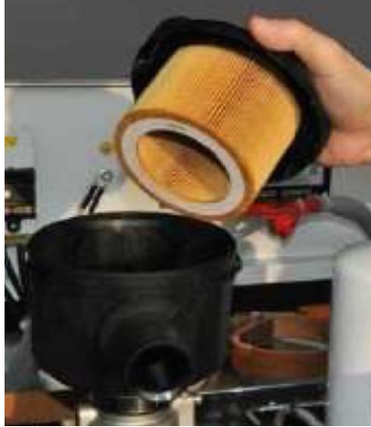
Figure 2-3 Air intake system
