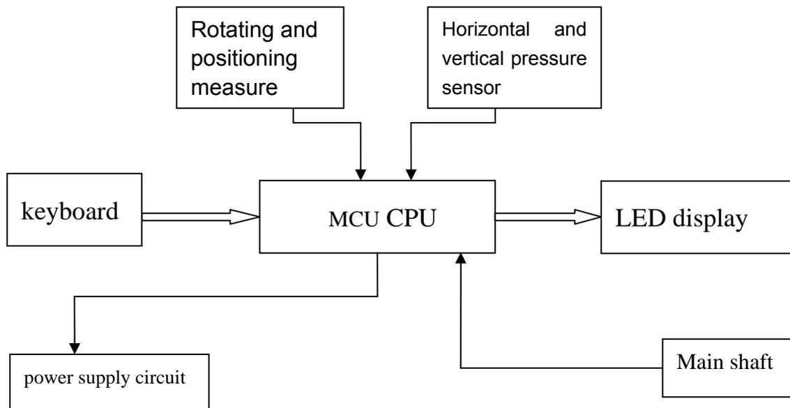
Fig 3-1 Electric system figure
