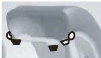
As per Fig 7-8 or Fig 7-9, move scale to rim inside (aI position ), measure rim inner distance (aI) value, press [a-] or [a+] to input aI value
