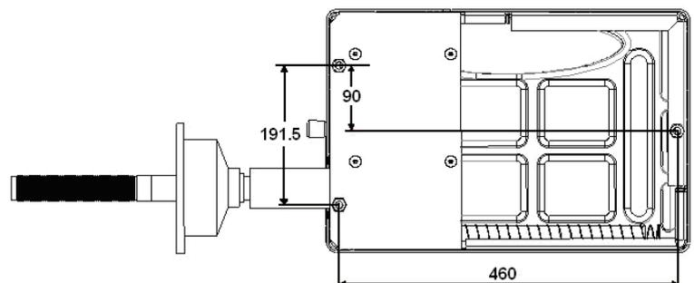
Installation holes position (bottom view)
